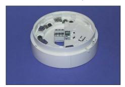
The 801RB provides dual relay contacts for signalling external devices on MX addressable systems. A very low operating current even when the relay is energised enables the relay base to be used without any additional power. The dual contacts are under the control of a programmable output, through the powerful cause and effect software.
