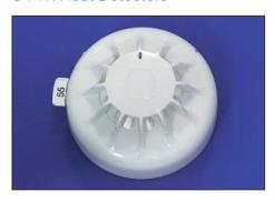
The 811H is a flexible cost-effective addressable heat detector with all the features of MX VIRTUAL detectors. The 811H returns the temperature to the MX detection panel which allows various detection modes to be implemented. The 811H uses a high quality thermistor with very low thermal mass. This allows the detectors to provide fast accurate temperature detection as well as heat detection.
