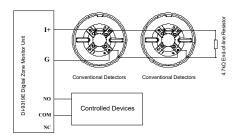
If the NO and COM terminals do not connect the controlled device, the DC24V power supply on the controller is needed, the system connection is shown as below.
