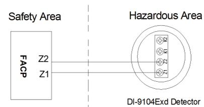
Below figures show the terminals and connection of the detector in non-addressable mode.
