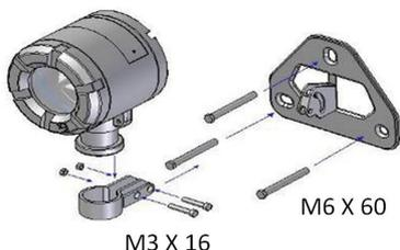
The detector should be installed facing the possible fire risk area, with calculated protection distance and space.
