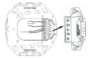
The access holes are provided in the back of the terminal block to allow the voltage to be measured directly without removing the device. Typically this would be done at the end of the line to confirm design criteria. Most measurements will be taken using the S+ and S- locations although access is provided to other locations. Note: Care should be taken not to short the test probes.
