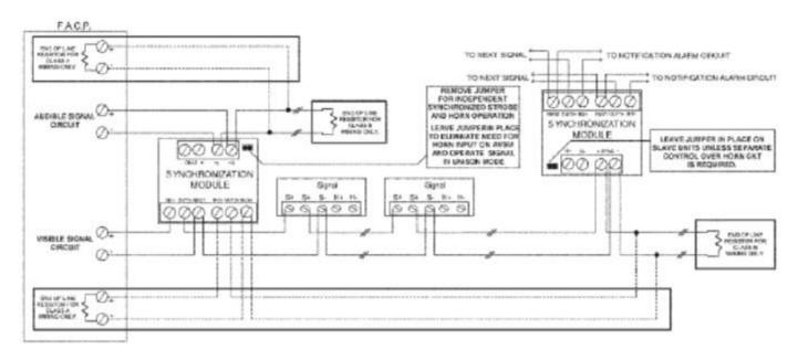
Wiring Diagram GCS/GCC Series With Gentex Synchronization Module
